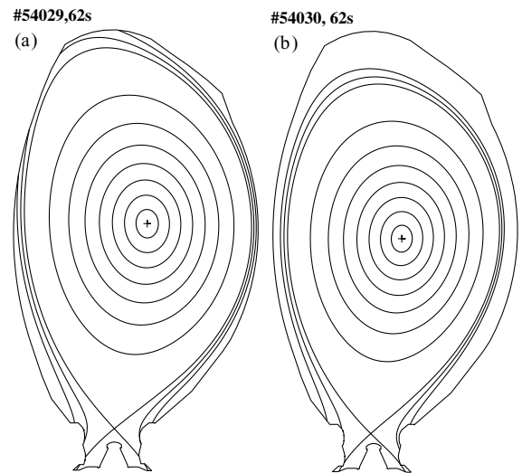
Fig. 1. Low (a) and high (b) wall clearance equilibria used for the majority experiments described in this paper.
